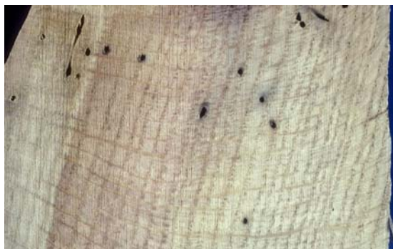
Platypus bore holes in oak heartwood with dark staining caused by ambrosia fungi
