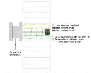
Figure 5. Partial inversion by the side strip method
