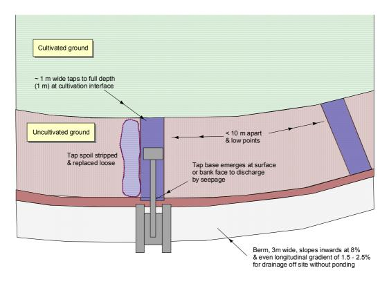
Figure 8. Drainage tap plan (example meets drainage berm)
