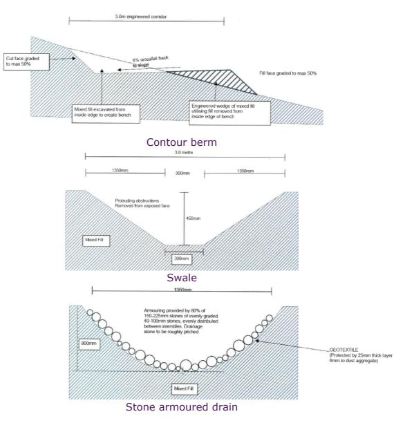
From Forestry Commission Scotland Schedule 'B' - Detailed specification for ground preparation and drainage works for the establishment of community woodland on a restored inert landfill at Greenoakhill, Broomhouse, Glasgow, January 2011. After Bending, N. & Waters, G. (2011).
