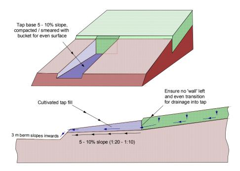
Figure 9. Drainage tap view (example meets drainage berm)
