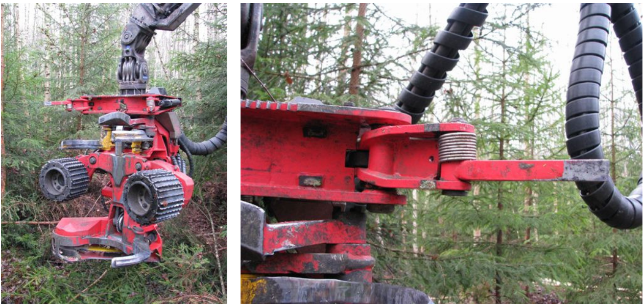
Figure 7. Accumulating arms holding cut birch.
