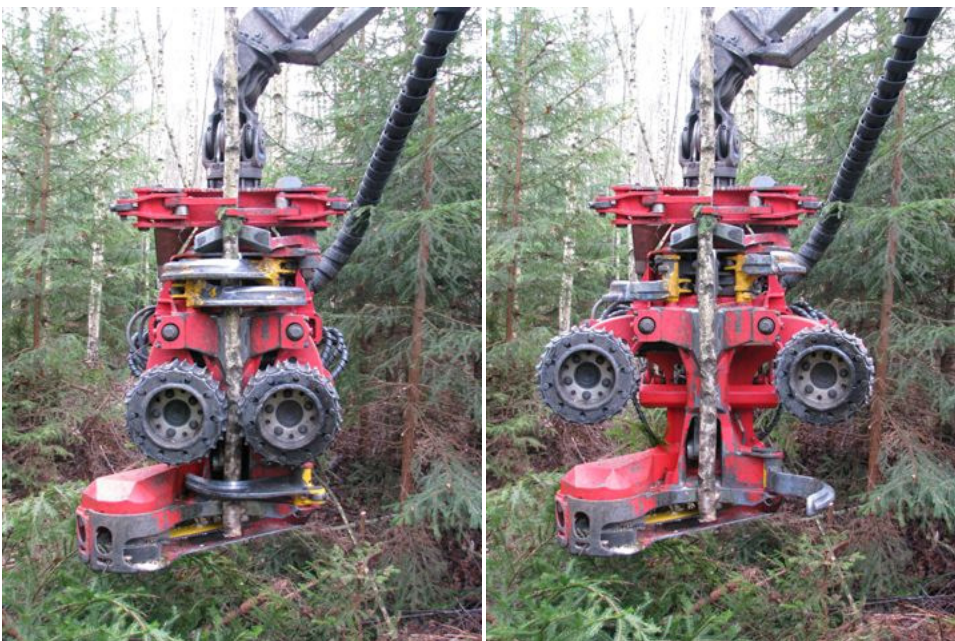
Figure 7. Accumulating arms holding cut birch.
